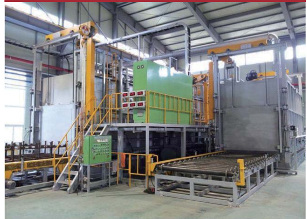
Heat treatment Continuous furnace with automatic system
